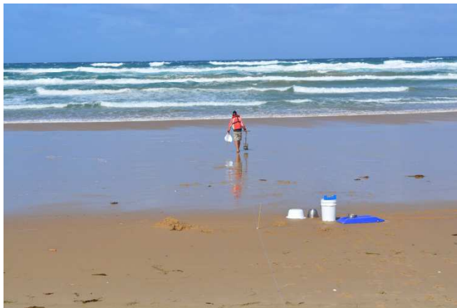
Surveying a beach transect. Note the corer in Fletcher's hand used to take standardised sand samples.
